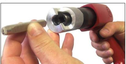
the stamp while actuating the trigger. When the trigger is pulled, a series of hammer blows "Burp" will create the mark. A one second "Burp" is all that is required. The stamp face may be inserted back into its indentation and a second "Burp" of the tool can create a deeper impression if desired.
